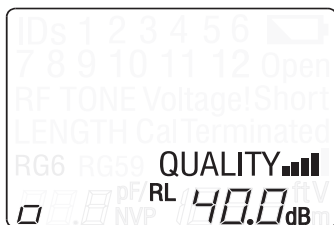
Figure 6. Return Loss Measurement in Quality Mode
